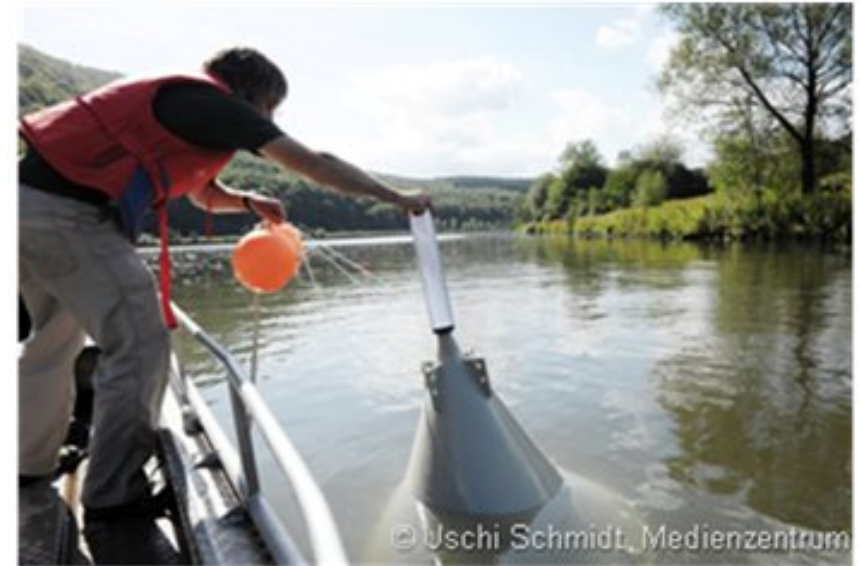
Measurement of upcoming methane-bubbles in the river Main by Universität Koblenz-Landau
